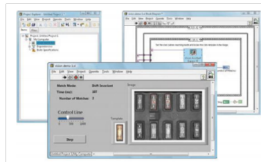
Figure 2. LabVIEW Front Panel, Block Diagram, and Project Explorer in a Vision Development Module Application
